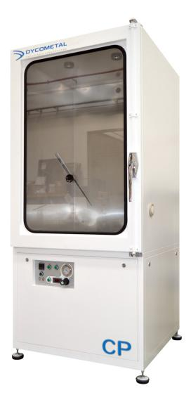
CP series are chambers designed to make aspiration, suspension or dust circulation tests, by exposing the sample to the study of the resistance of dust penetration on its moreless tight structure.
